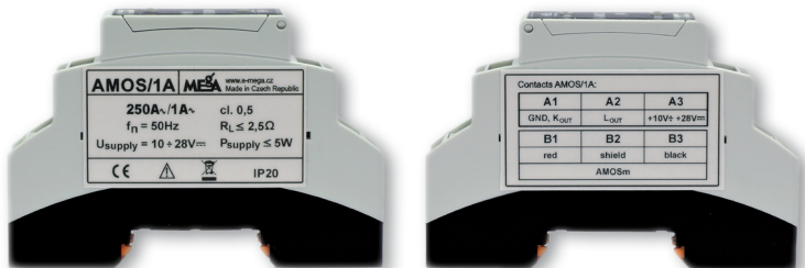
Fig. 1: Data label and a label displaying the connecting of contacts of the AMOS/1A converter unit
